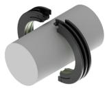
The seals can be installed before or after the radial and axial bearings are assembled. If fitted before the bearing, slide the seals axially away from each side of the bearing position allowing space to assemble the bearing.
