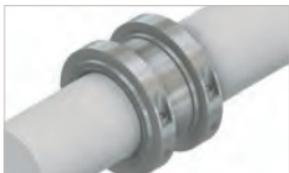
For expansion bearings, the inner race can be offset according to the amount of shaft thermal expansion, so that when operating temperature is reached, the rollers will run central to the outer race. When fitted, re-check the inner race and clamp ring joint gaps are equal and the race is correctly positioned axially.
